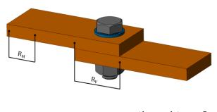
figure of merit  $k_u = \frac{\text{connection resistance } R_v}{\text{material resistance } R_M}$
